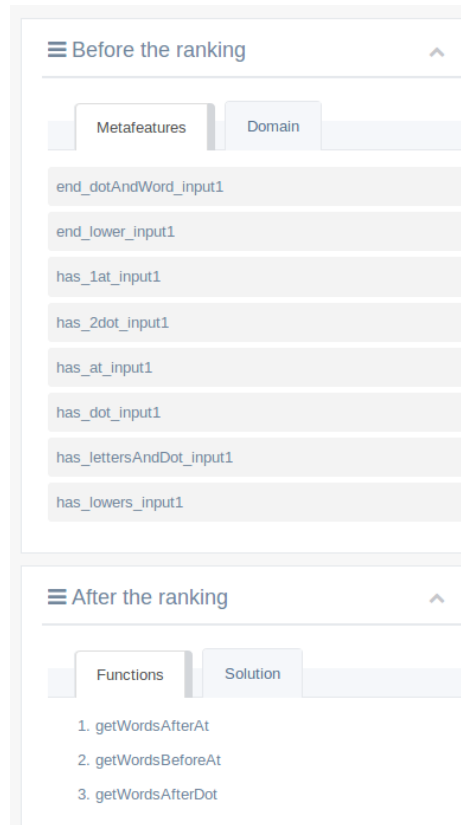
Figure D.3. The system shows to the user the list of meta-features extracted from the examples and the background knowledge generated.
